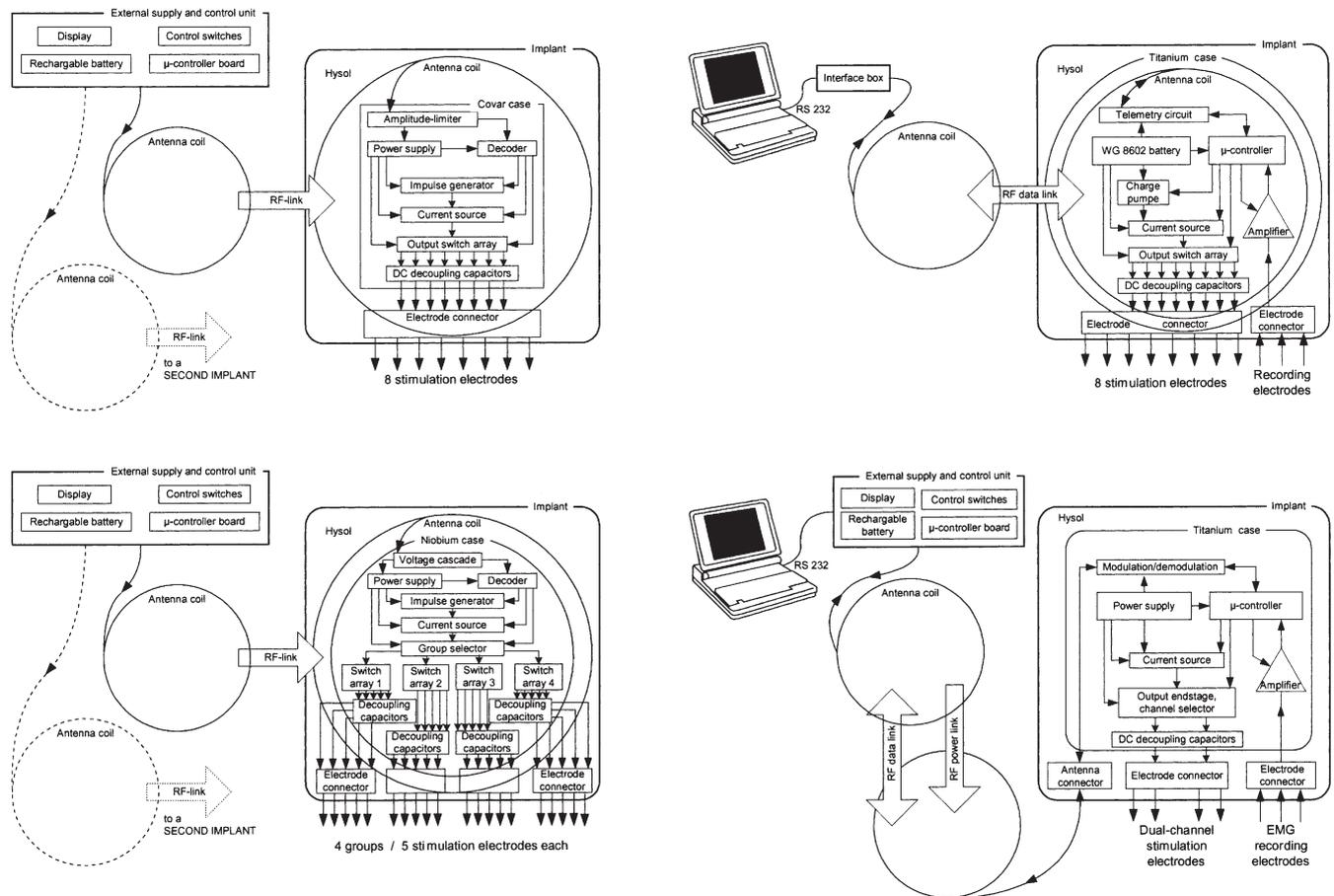
Fig. 3. Schematic diagram of all 4 Vienna implants: Left side: RF-powered 8-channel and 20-channel implant, Right side: Battery powered 8-channel implant and RF-powered 2-channel implant for denervated muscles.
