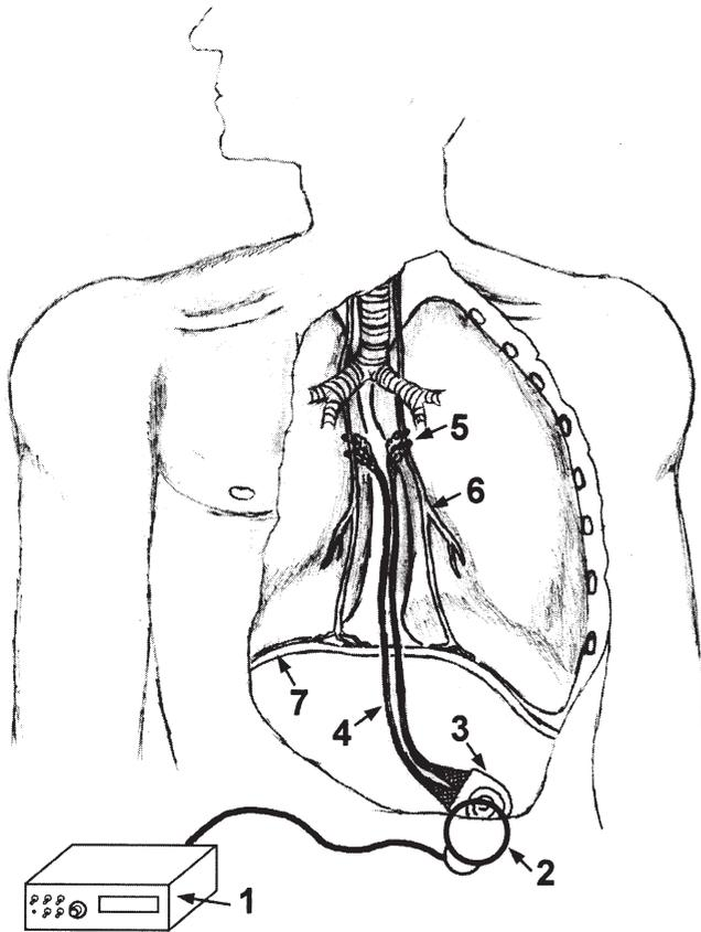
Fig. 2. The phrenic pacer, designed to elicit respiratory movements of the diaphragm in cases of high level injury to the cervical spinal cord or central hypoventilatory apnoea (Ondine's curse). (1) External supply and control unit; (2) Transmitter; (3) 8-channel implant; (4) Electrode leads; (5) Epineural electrodes; (6) Phrenic nerve; (7) Diaphragm.
