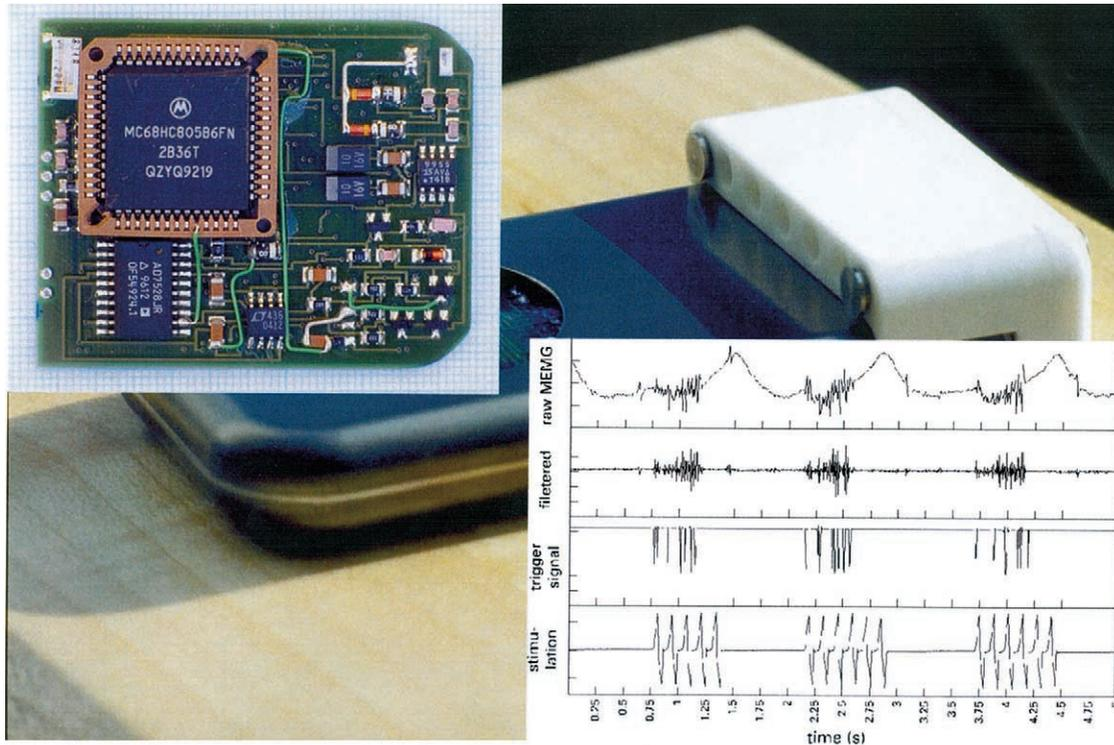
Fig. 4. Prototype version of the RF-powered EMG-controlled 2-channel implant for denervated muscles: Left side: SMD-circuit, Right side: Recorded and processed diaphragm EMG and stimulation impulse, Background: Hermetic titanium case and connector unit made from oxide ceramic.
