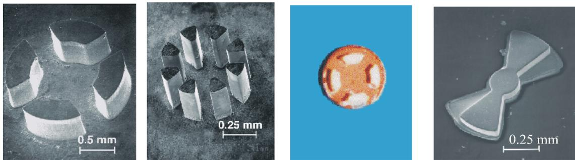
geometry can be approximated by stacking sufficiently thin 2D layers. A copper micro-propeller approximated by two-layer silicon mold is shown in Figure 7.
