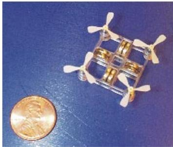
**Figure 1** Prototype of 16mm x 16mm Mesicopter.
