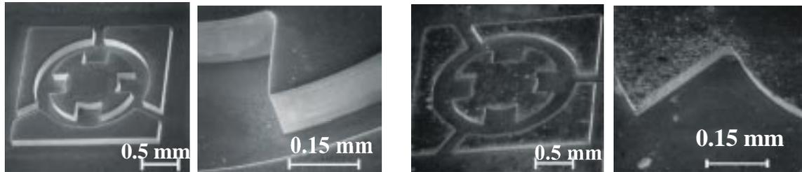
MPa for one hour. This temperature and pressure setting was low enough to avoid plastic deformation of the silicon. The final AgW part has around 93% of the theoretical full density, and replicates the mold sufficiently well (Figure 9).
