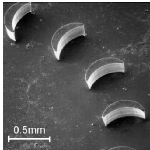
Fig. 6 SEM picture of an herring-bone bearing pattern generated by photolithography with SU-8 50 (Left) ; gel-cast ceramic green body fabricated with SU-8 PR mold (Right).
