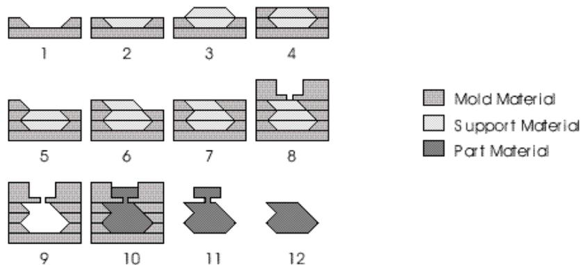
Fig. 2 Schematic representation of the Mold SDM process: the mold is constructed layer by layer. After that, the support material is dissolved and the ceramic part is gel-cast.
