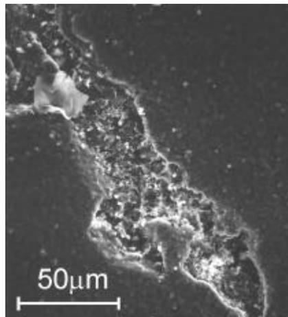
Fig. 3 Surface crack on the surface of the Mold SDM Si<sub>3</sub>N<sub>4</sub> specimen.
