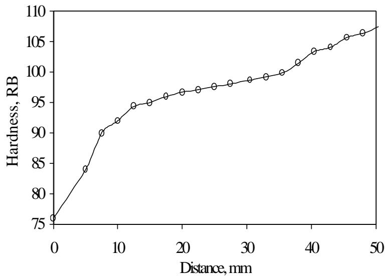
Figure 6. Hardness of Functionally Gradient Deposited Invar and TiC
