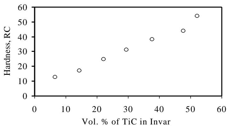
Figure 3. Hardness Test Results
