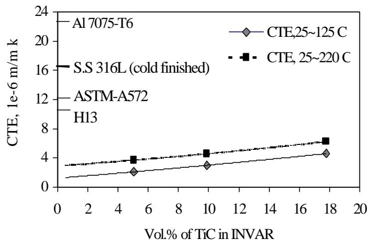
Figure 5. CTE of Composites in Comparison with Metals
