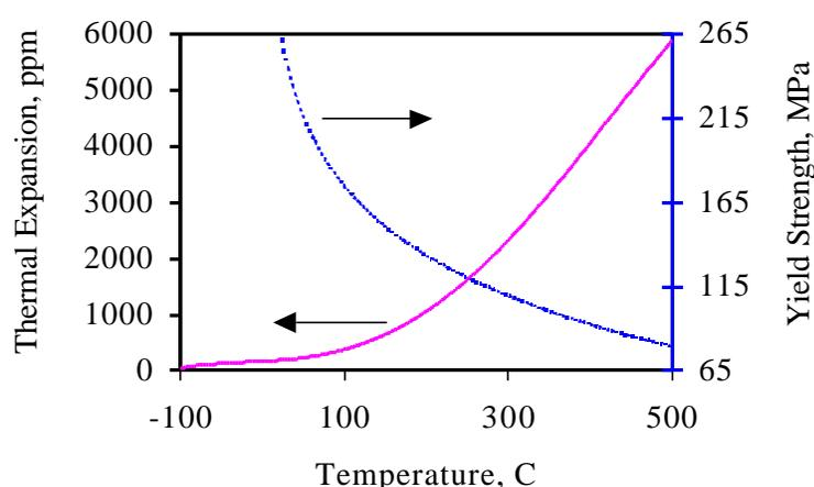
Figure 1. Thermal expansion and Yield Strength of Invar
