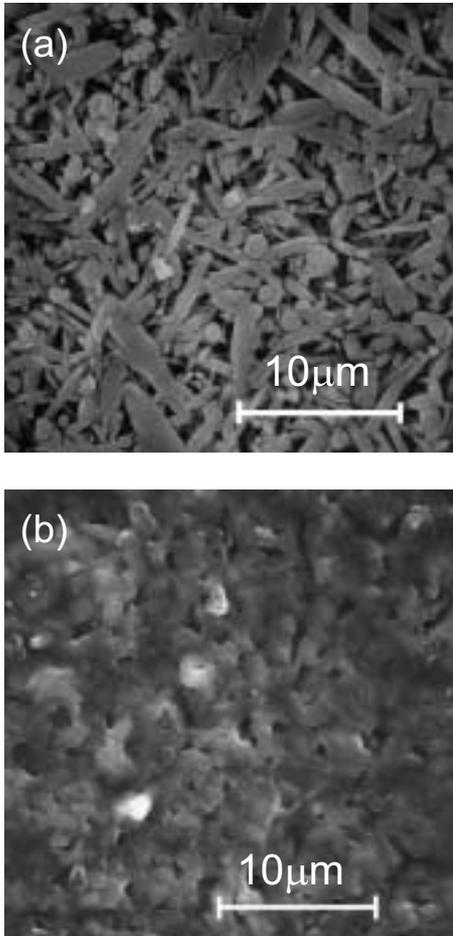
Figure 6: Microstructure of sintered silicon nitride in the bulk material (a) and on the surface (b).
