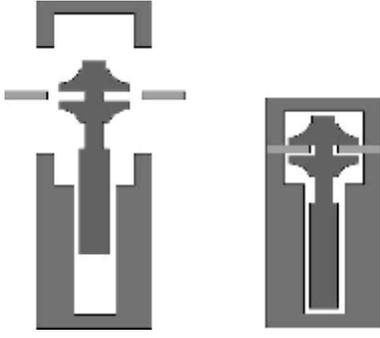
Figure 8: Sintering configuration for the silicon nitride rotor group to avoid distortion during sintering.
