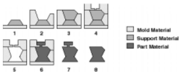
Figure 5: Mold SDM procedures
