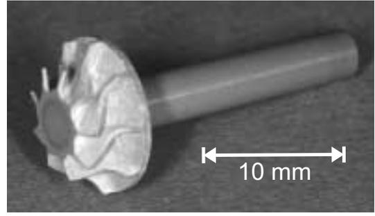
Figure 9: The sintered turbine shaft used for the spin test.
