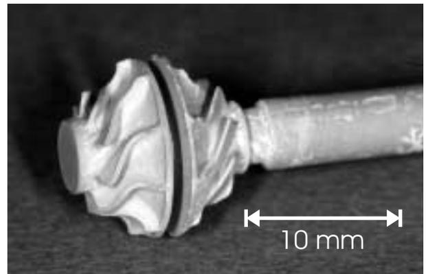
Figure 7: Sintered silicon nitride rotor group.
