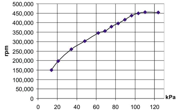
Figure 10: Spin test result of the turbine shaft geometry.
