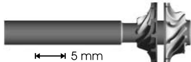
Figure 2: CAD model of the silicon nitride rotor group of the micro gas turbine engine.
