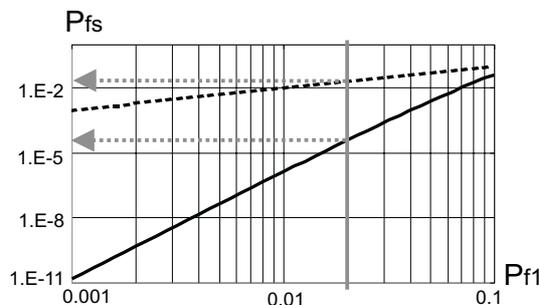
Figure 4: The failure probability comparison of one big engine engine (dotted black line) and 20 small engines (solid line) system.  $P_{f1}$ : failure probability of each engine,  $P_{fs}$ : failure probability of 20 engine system
