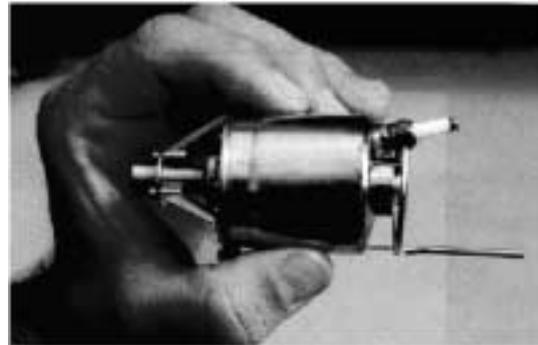
Figure 1: M-DOT micro gas turbine engine
