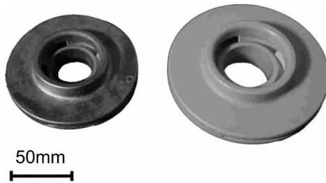
Fig. 5. Sintered stainless steel impeller (left) and polyurethane impeller (right).
