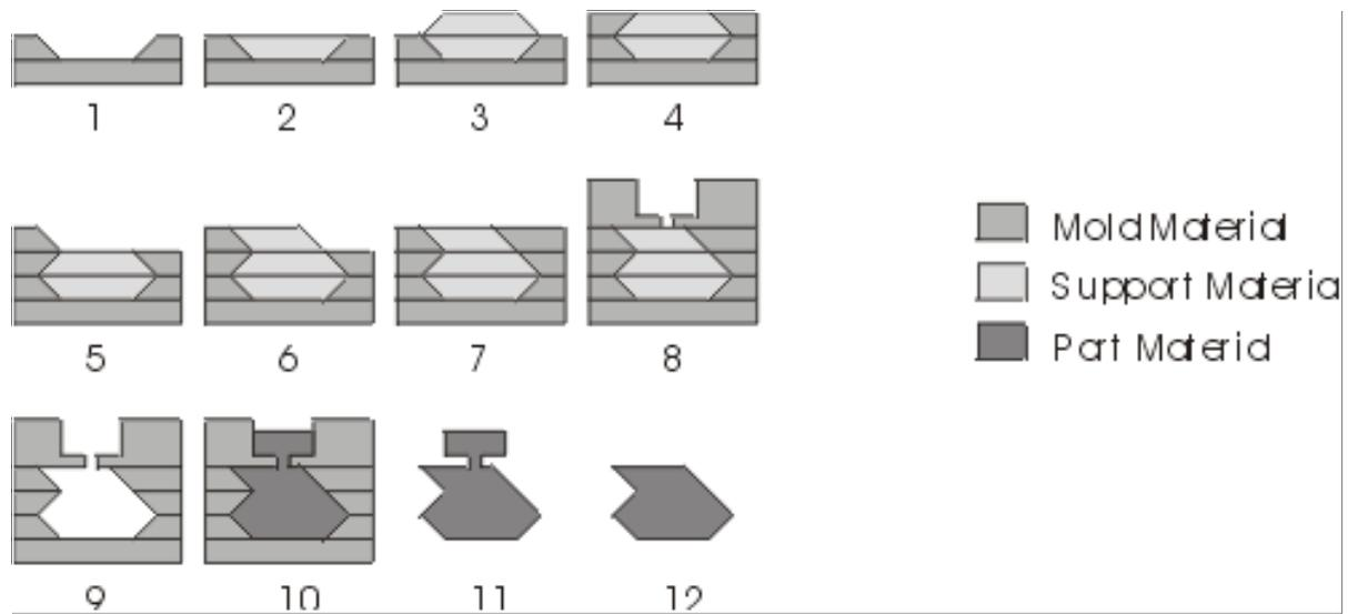
Figure 1: Example Mold SDM process sequence
