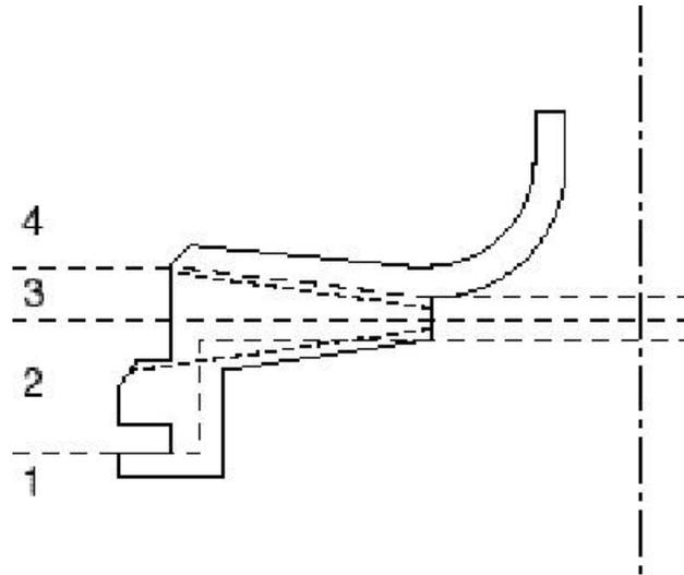
Figure 8: Inlet nozzle decomposition
