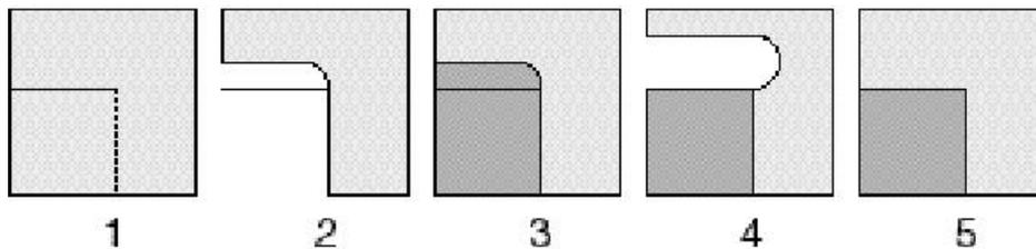
Figure 9: Sharp corner fabrication technique
