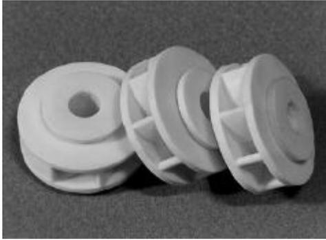
Figure 2: Alumina turbine
