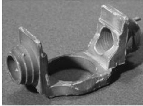
Figure 3: Silicon nitride pitch shaft
