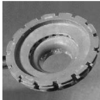
Figure 11: Sintered inlet nozzle
