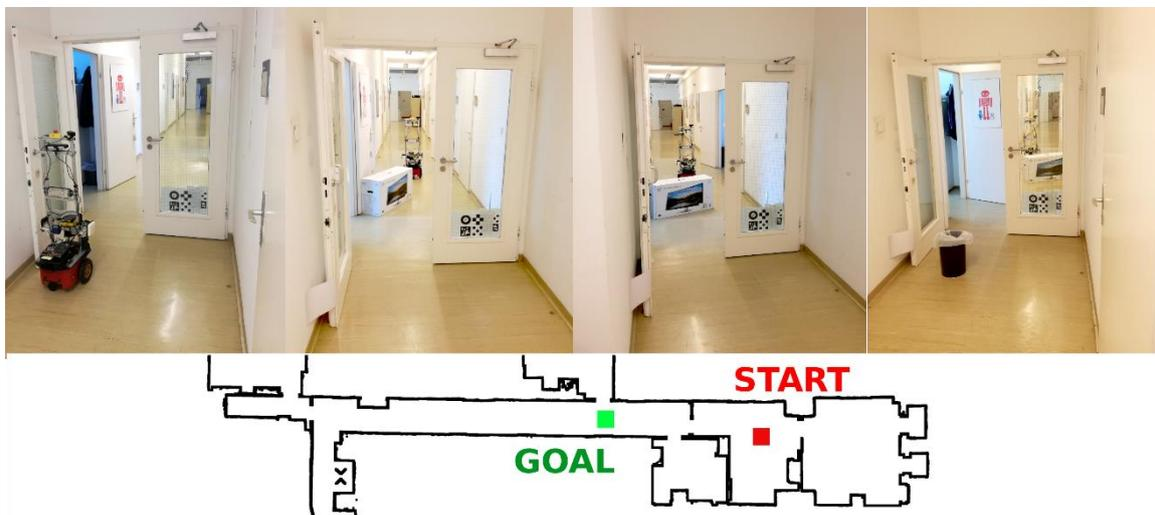
Fig. 6: Four test scenarios from, left to right: no obstacle, easy obstacle, hard obstacle, hard environment and corresponding map with start and destination (goal) positions.
