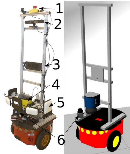
Fig 2: The real and simulated Pioneer 3DX robot used for experiments. 1 - emergency stop button, 2,3 - depth cameras, 4 - SICK Laser scanner, 5 - AirSkin, 6 - Hokuyo laser scanner
