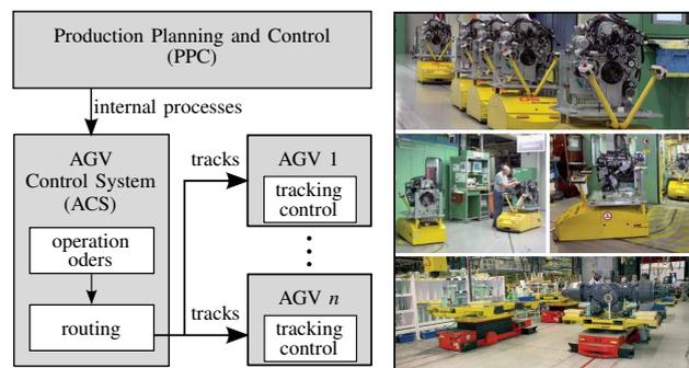
Fig. 1. This figure shows, to the left, the modules involved in a classical system. The PPC analyses general processes (e.g., customer requests) for the ACS. The ACS identifies operation orders in internal processes and computes routing tables composed of sequences of line, arc and spline segments as tracks. A single AGV has to simply follow the tracks with a tracking control. No path planning is involved. To the right, AGVs in action on an automotive assembly line.
