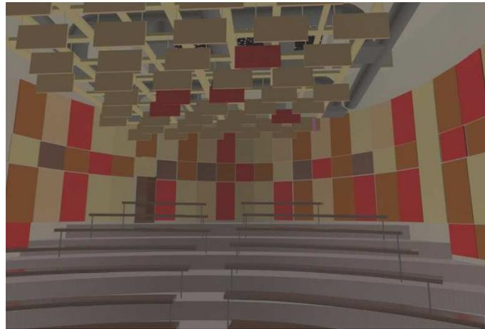
Use of baffles under the skylight and rear wall.
